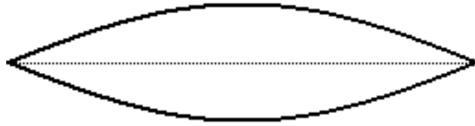
A plucked string vibrating in its fundamental resonant mode
